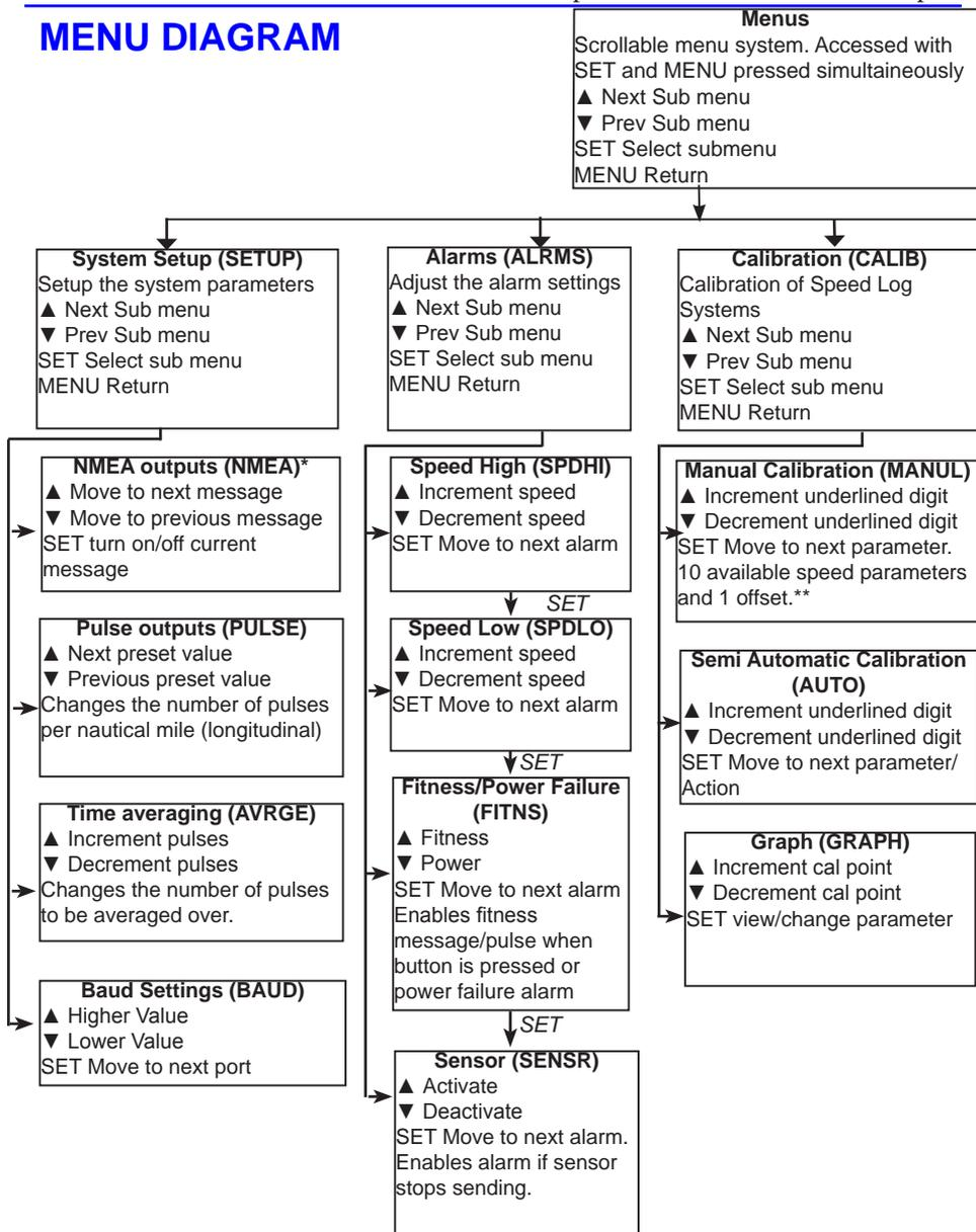
\* One option in the NMEA settings is DIAG. This turns on some of the diagnostics outputs. These are propriety messages that occur if an error occurs or if requested. Setting this to 'ON' will stop all other messages.
