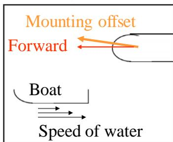
Full calibration is designed to ignore water current effects. The procedure requires the vessel to sail a fixed length track, at a constant speed. To remove the current and
