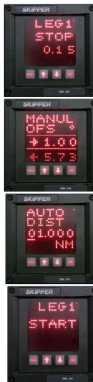
**Note:** The user should press the start and stop based on position on the chart, and not sailed distance on the unit..
