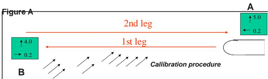
If necessary, the procedure should be repeated at different speeds. SKIPPER recommend that calibration is performed at a low speed and a high speed. If the user is not able to turn the vessel and is sure there is no current, the calibration procedure can be stopped after the first leg and saved as a calibration point.
